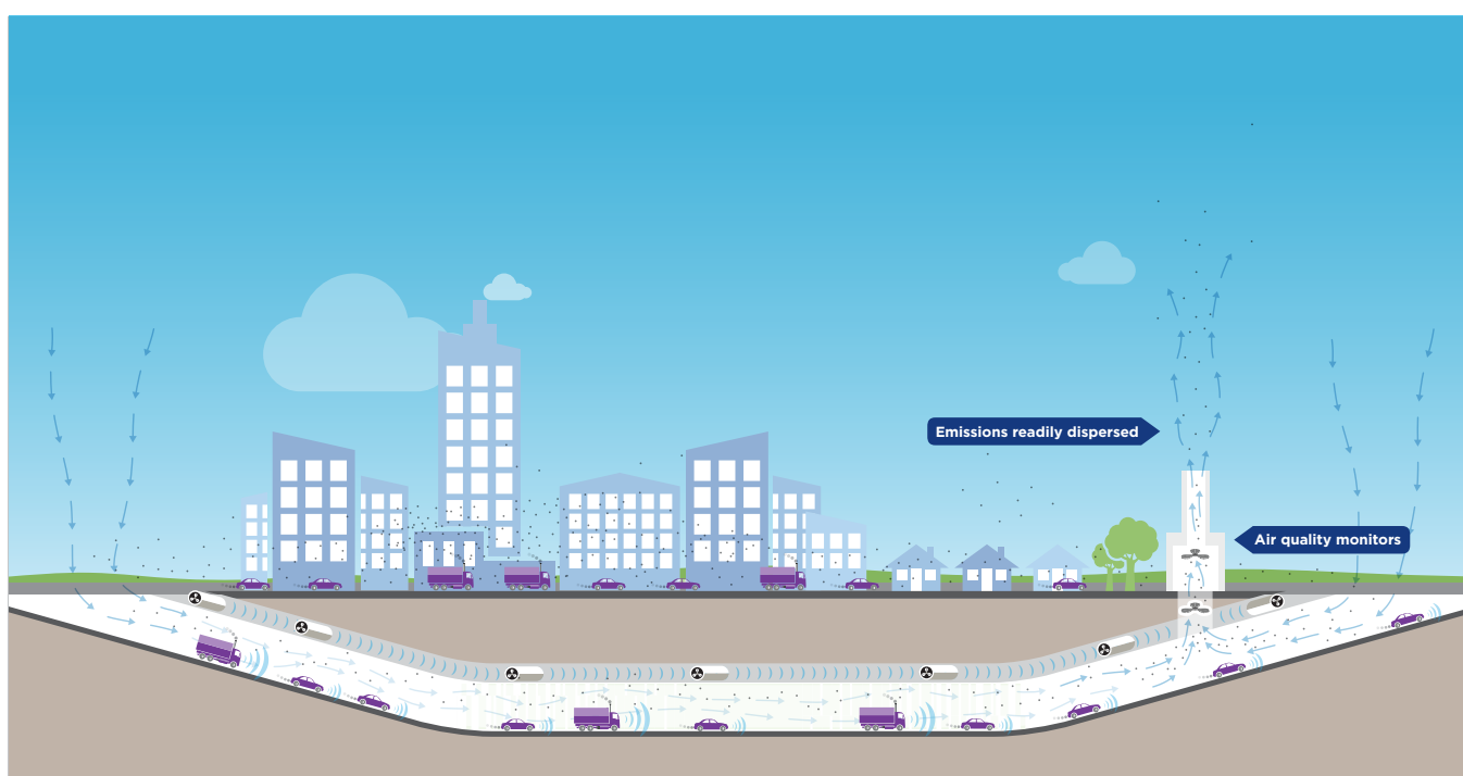
Artist's impression of longitudinal tunnel ventilation system.
